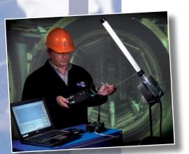
The Datapaq<sup>®</sup> Q18 radio telemetry system utilizes the latest radio-frequency technology to allow data transmission from the data logger in real time. As the Datapaq system travels through the process, product and process temperature data can be viewed, analyzed and reported instantaneously. This technology can be applied to monitoring key thermal processes in most industrial heating applications.
